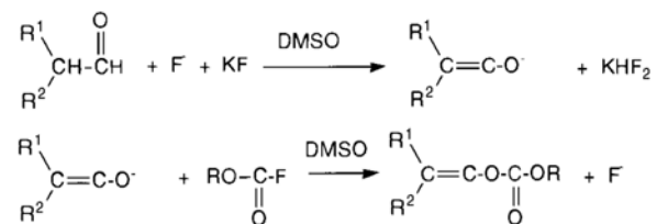
Scheme 99 : Mechanism of the reaction of fluoroformates with aldehydes in presence of KF in DMSO.
